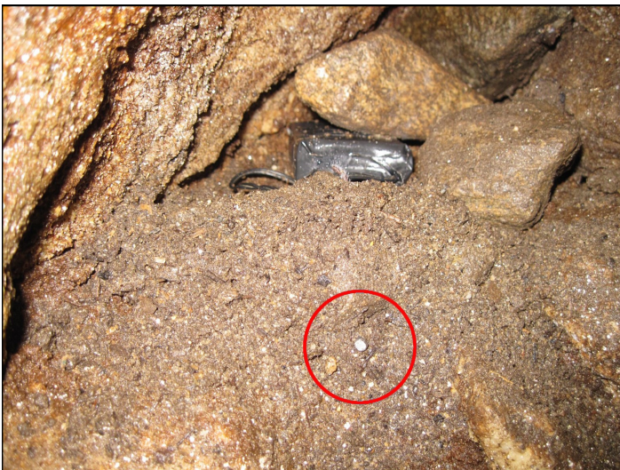
Stages in sensor placement within the cave. The case housing the electronics and wires are carefully buried and concealed (left) so that only the sensor is exposed (right). Only about 1/8 inch in diameter, the sensor looks much like other shiny crystals in the cave wall and is largely invisible to anyone passing near it. Photos by Norm Berg.
