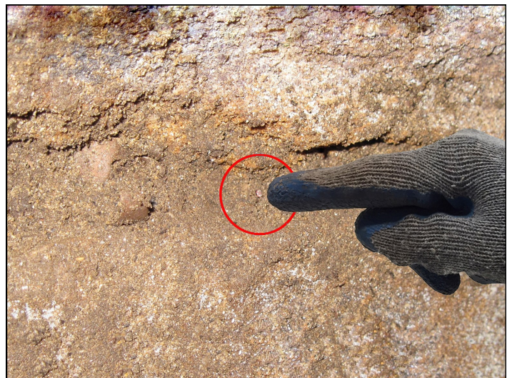
Stages in sensor placement within the cave. The case housing the electronics and wires are carefully buried and concealed (left) so that only the sensor is exposed (right). Only about 1/8 inch in diameter, the sensor looks much like other shiny crystals in the cave wall and is largely invisible to anyone passing near it. Photos by Norm Berg.
