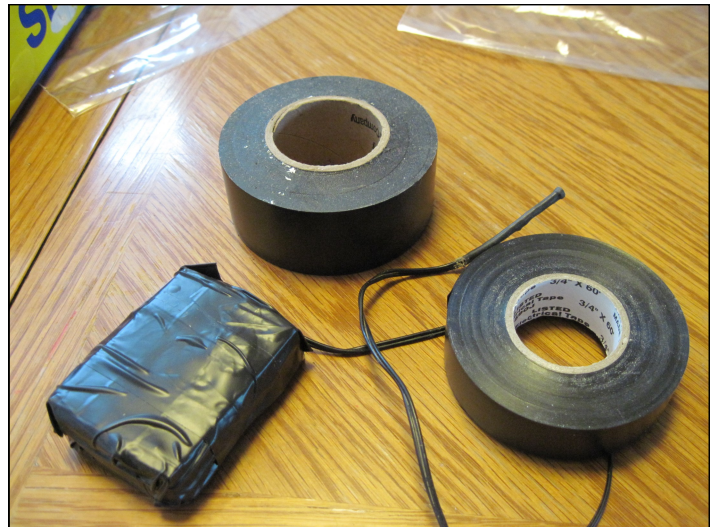
Preparation of logger to survive the cave environment includes wrapping the logger in inner (left) and outer (right) protective layers. The layers help waterproof the logger, protect it against abrasion, and help to camouflage it. Data collection by the logger actually begins before it is wrapped. However, data not relevant to the study is discarded prior to analysis. Photos by Norm Berg.
