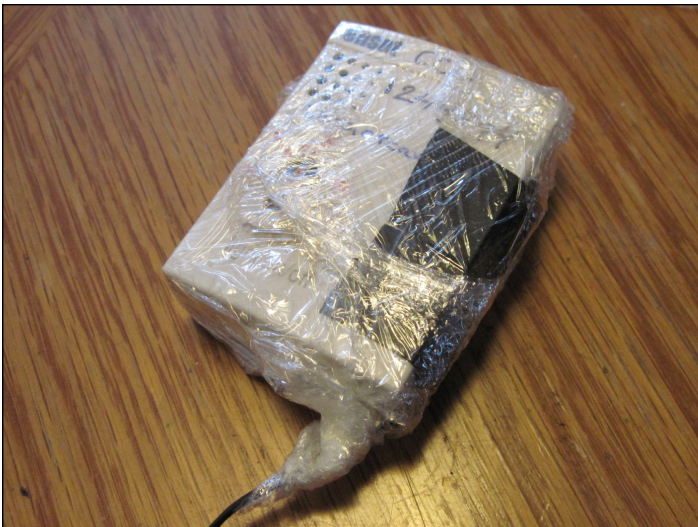
Preparation of logger to survive the cave environment includes wrapping the logger in inner (left) and outer (right) protective layers. The layers help waterproof the logger, protect it against abrasion, and help to camouflage it. Data collection by the logger actually begins before it is wrapped. However, data not relevant to the study is discarded prior to analysis. Photos by Norm Berg.
