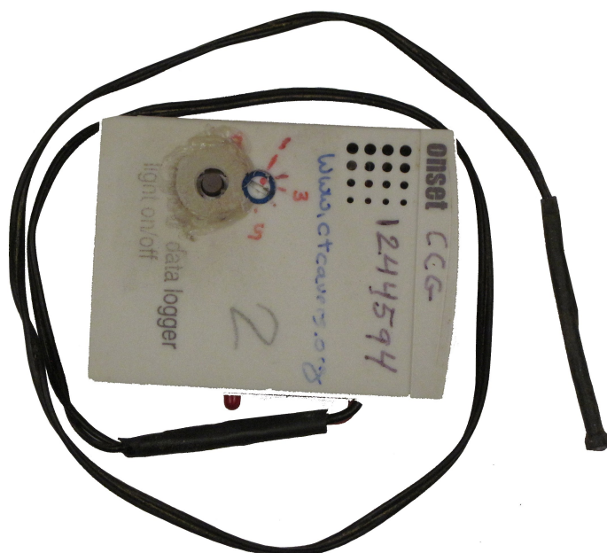
The Hobo U9-002 Light On/Off data logger modified for use in a cave environment. Photo by Norm Berg.
